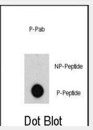
Dot blot analysis of anti-ABL-pY185 Pab (RB07973) on nitrocellulose membrane. 50ng of Phospho-peptide or Non Phospho-peptide per dot were adsorbed. Antibody working concentrations are 0.5ug per ml.
